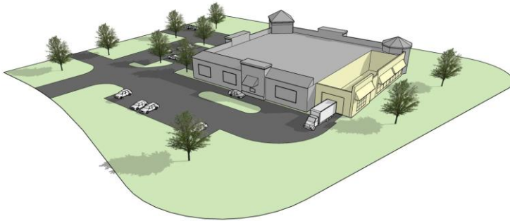
Figure 1204.14-1 Illustrative Example of Enclosed Loading
