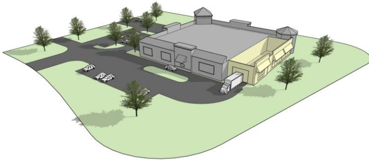
Figure 1204.14-1 Illustrative Example of Enclosed Loading
