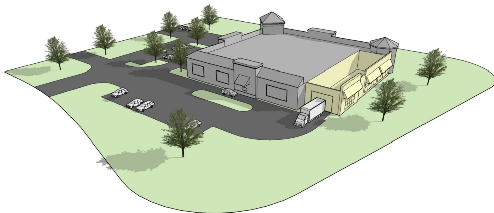
Figure 1204.14-1 Illustrative Example of Enclosed Loading
