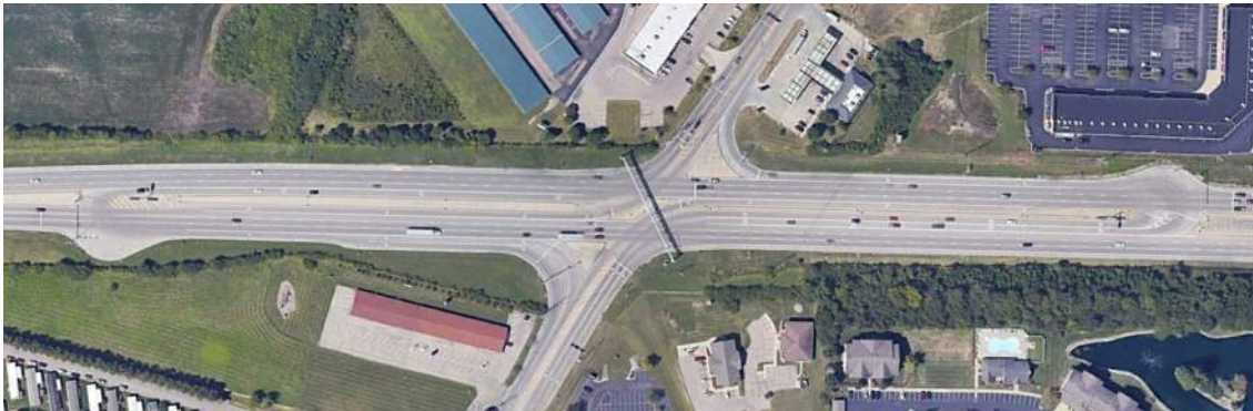
Figure 7: Example RCUT Intersection in Hamilton, OH
