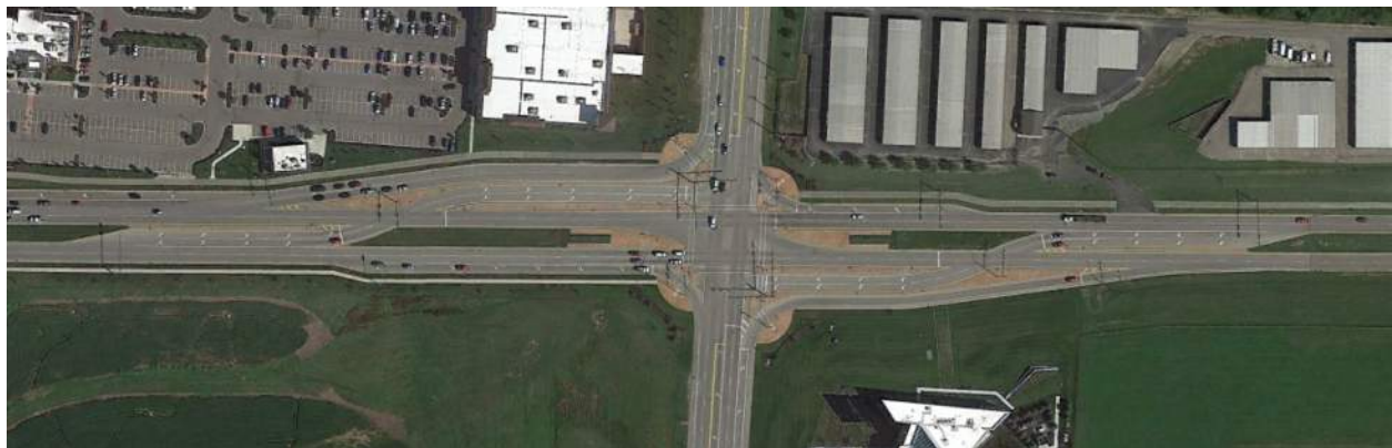
Figure 9: Example Partial CFI/DLT in Miamisburg, Ohio
