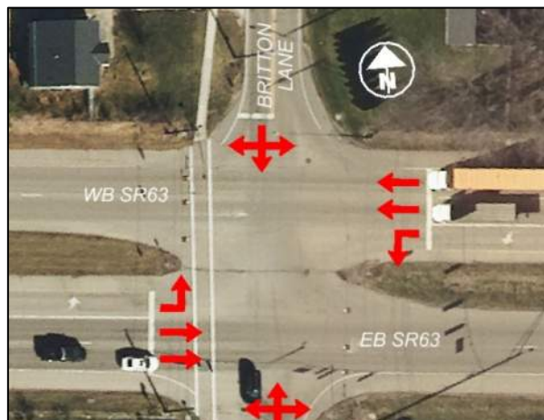
Figure 2: Britton Lane & SR 63 Lane Configuration
